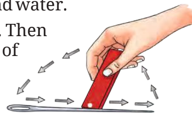
Fig. 4.7(a): Making an iron needle a magnet
