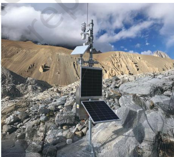
Fig. 2.12. AWS at a glacial lake of Sikkim
