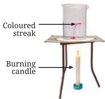
Fig. 7.5(b): Demonstration of convection in heated water
