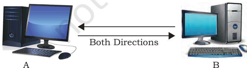
Figure 11.5: Full duplex transmission of data
